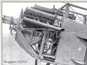
Engine bay detail from 79 Squadron early production Sopwith built Dolphin C3905 which was captured on 23 March 1918 and extensively examined by the Germans. Note the gears of the Constantinesco (CC) synchronizing system (A25). This photo and all following photos show 200hp Hispano-Suiza V8 geared "Hisso" powered Sopwith SF1 Dolphin 1 unless specified otherwise.
