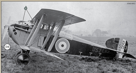
Late production Sopwith 5F.1 Dolphin D5263 is from a production order for 200 aircraft placed with Hooper & Co Ltd in June 1917 (numbers D5201 to D5400) but does not appear to have been completed until very late 1918. Note the very pale battleship (service?) grey interplane struts (1) and how the matt black serial number on the fuselage appears paler than the gloss PC10 because of how it is reflecting the light. Also note the very late production front cowl (D8).
